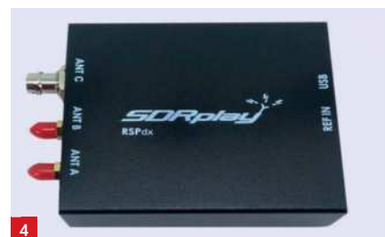
Fig. 1: No MW-Amore anymore: RAI Radio Italy has left Medium Wave. Fig. 2: WFED Federal News Radio. Fig. 3: The Tecsun PL-990x World Band Receiver. Fig. 4: The SDRplay RSPdx Software-Defined Receiver enables users to record the bands overnight and catch up the next day.
