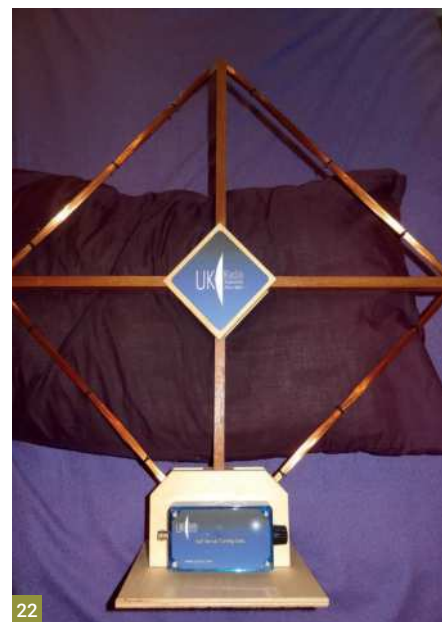
Fig. 20: The day's best results on the Reuter RLA3 . Fig. 21: Clearer reception of the same range with the BAZ Ferrite Bar LFM/S1-N (see also Fig. 8 in Part One). Fig. 22: The assembled UKRAA Loop and Aerial Tuning Unit (ATU) attached to it.
